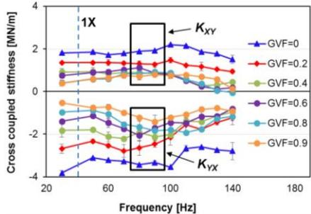
**Fig 4. Seal cross coupled stiffnesses vs. frequency ( $\omega$ ). Journal speed 2.5 krpm.**
