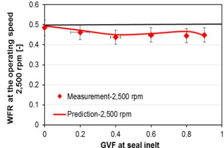
**Fig 5. Whirl frequency ratio (WFR) vs. inlet gas volume fraction. Journal speed 2.5 krpm.**
