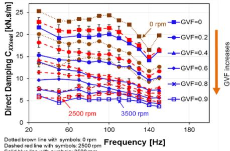
**Fig 3. Seal direct damping ( $C_{xx}$ ) vs. frequency ( $\omega$ ). Journal speed: 0 rpm to 3.5 krpm.**
