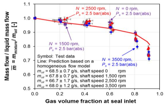
Fig 2. Mass flow rate vs. inlet gas volume fraction. Supply / discharge pressure  $P_s / P_a = 2.5$ . Inlet temperature  $T_{in} = 33$  °C -35 °C. Journal speed 3,500 rpm ( $\Omega R = 23.3$  m/s).
