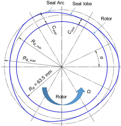
**Fig 6. Wavy seal schematic view:  $D = 127\text{ mm}$ ,  $L = 46\text{ mm}$ ,  $c_{max} = 0.244\text{ mm}$ ,  $c_{min} = 0.163\text{ mm}$ ,  $c_{ave} = 0.203\text{ mm}$ .**
