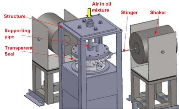
Fig 1. Side view of the seal test rig
