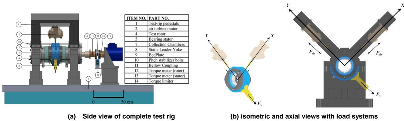
Figure 1. Schematic views of fluid film bearing test rig.
