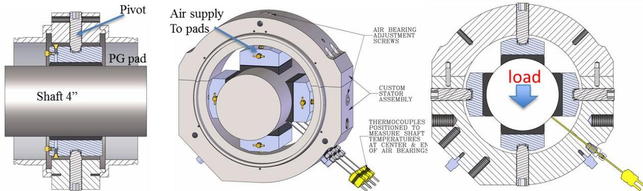
Fig. 2 4-pad porous Carbon-Graphite tilting pad gas bearing designed for ready test in existing facility.
