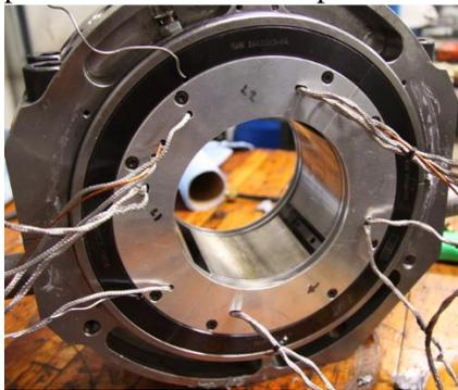
Fig. 2 4-pad bearing with spherical pivots and single orifice oil feed
