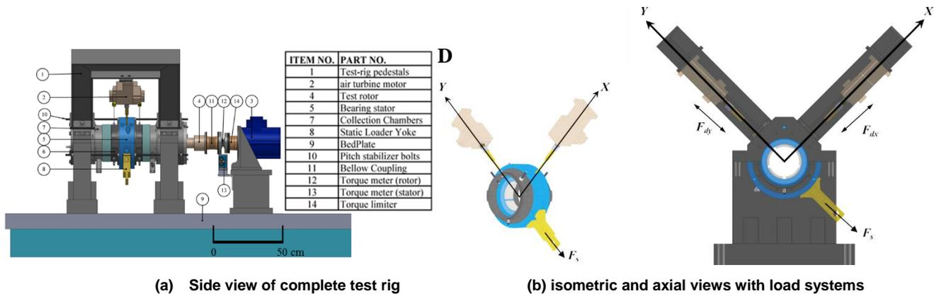
Figure 1. Schematic views of fluid film bearing test rig.
