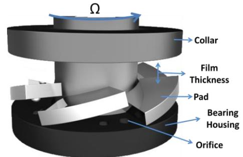
**Fig. 1: A schematic view of a 6-pad TPTB (exaggerated clearance)**
