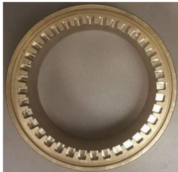
Figure 2. A swirl brake for an annular seal. Photograph from Ref. [3].
