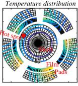
(b) **Dynamic Coefficients**: Accurate prediction of dynamic coefficients for tilting/fixed pad includes effect of 3D lubricant temperature, nonlinear pivot stiffness, 3D flexible pad model, misalignment effect, bearing structure deformation and 3D deformation of
