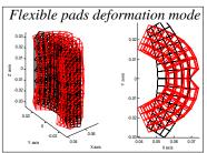
(h) 3D tilting pad bearing model with tilt-pitch-yaw of pad and nonlinear stress conditions (including axial) on pivot will provide more accurate predictions of pivot fatigue life.
