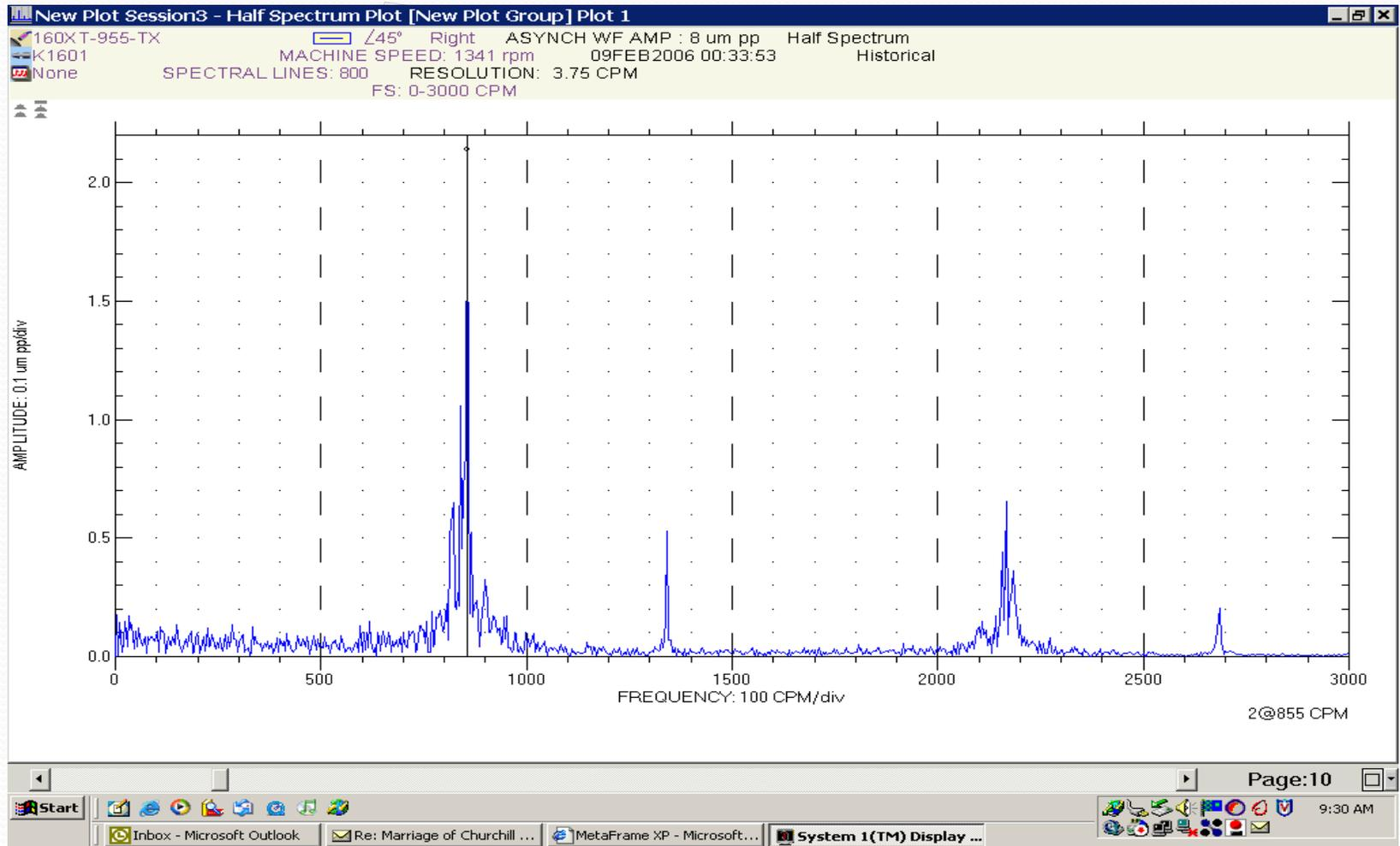
**Vibration spectrum on bull gear
