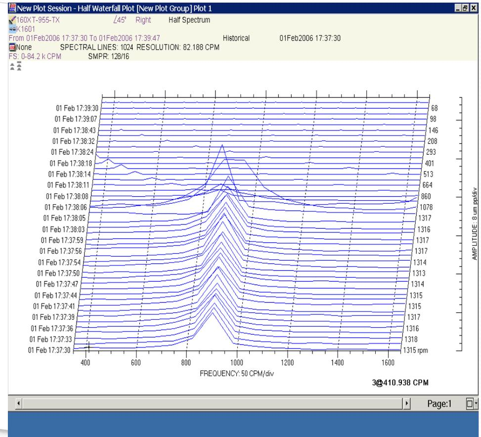
**Overall vibration plot with speed and coast down waterfall from hard stop**
