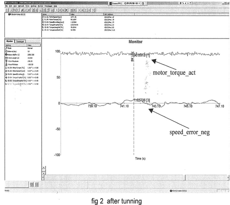
Motor torque and speed error before and after tuning
