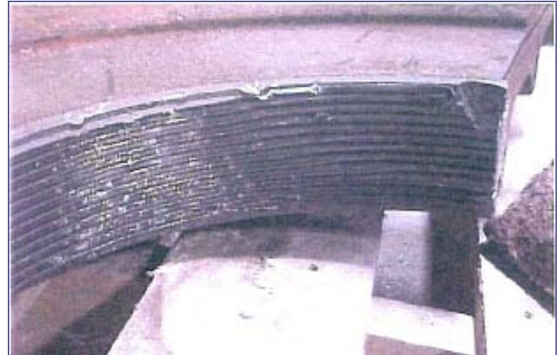
Mechanical Seal Damage
