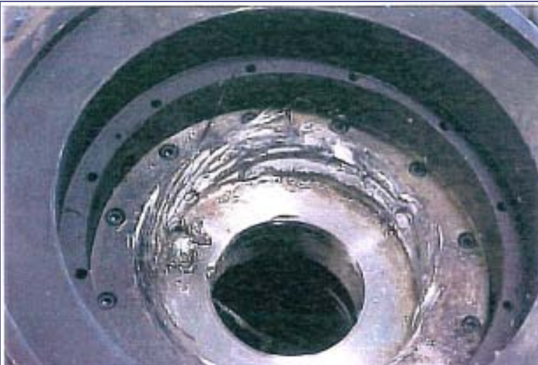
Bearing Housing Damage
