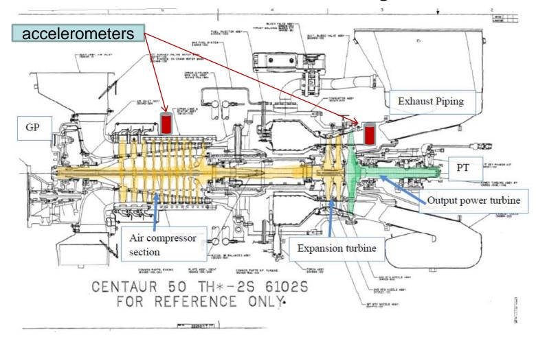
Output power turbine (PT) and gas producer (GP) are on separate shafts.Share common housing.
