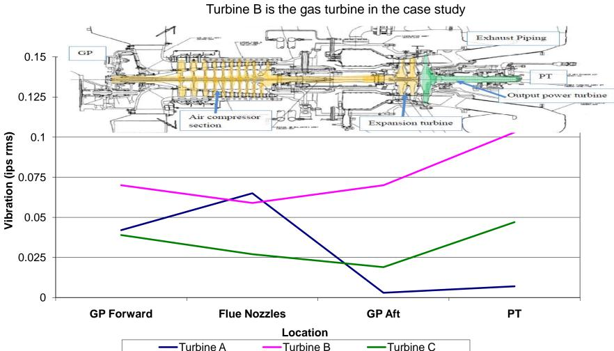
Gas Producer Vertical Vibration Levels at Different Train Locations
