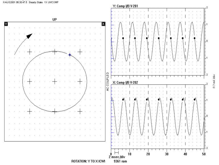
POINT: Comp I/B V-201 /45° Left DIR AMPL: 2.55 mil pp POINT: Comp I/B V-202 /45° Right DIR AMPL: 2.50 mil pp MACHINE: IP Compressor MACHINE SPEED: 9361 rpm
