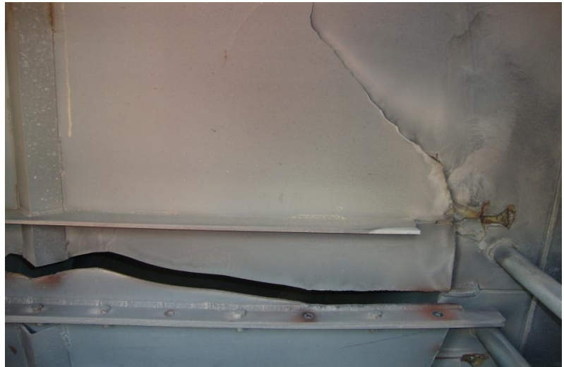
Casing internal damages / cracks
