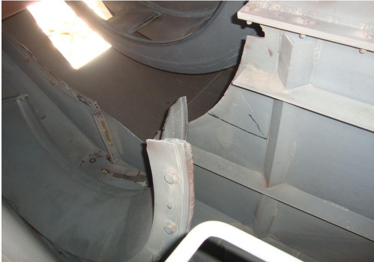
Casing internal damages / cracks
