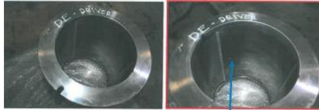
Main bearing Drive and driven side found with scratch marks.
