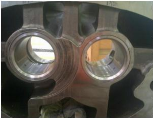
Damage casing (in conjunction to male rotor (see above pic)...
