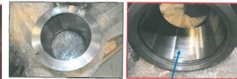
Side bearing Drive and driven side found with dents mark.
