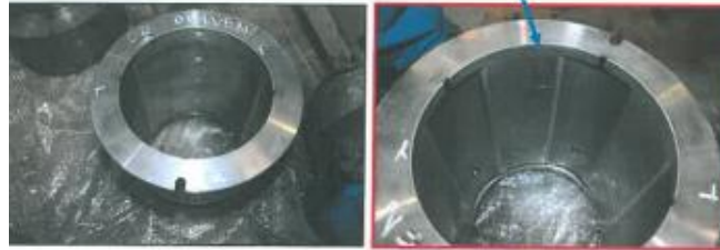
Main bearing Drive and driven side found with scratch marks.
