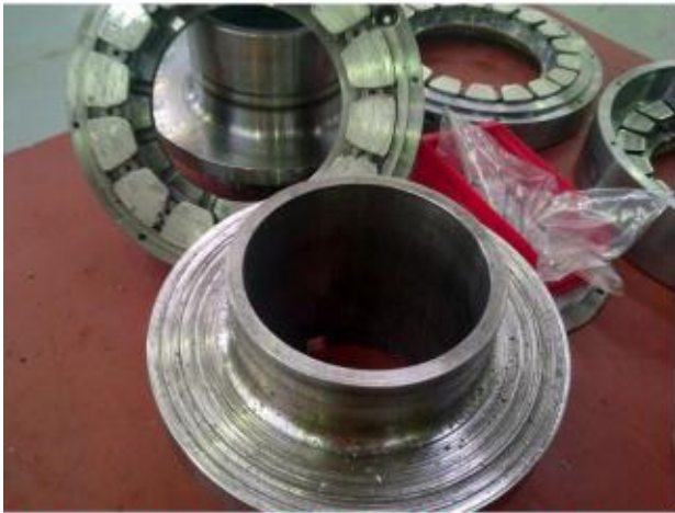
Thrust runner and thrust bearing of male rotor....
