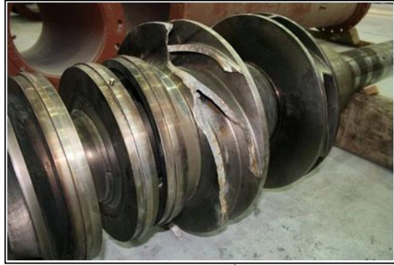
Figure 5: G-2001 new rotor 2 nd stage shroud breakage
