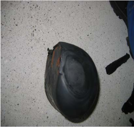
Figure 15. Overloaded Elastomeric Damper Element.
