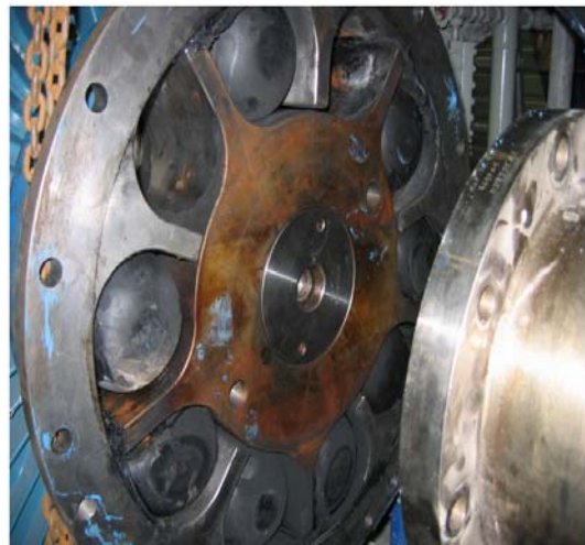
Figure 14. Overloaded Elastomeric Coupling.
