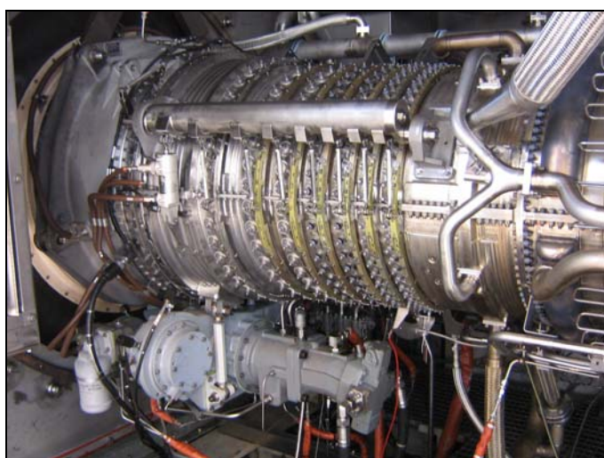
Figure 43. Gas Generator Showing Torque Tube for Variable Geometry Control.
