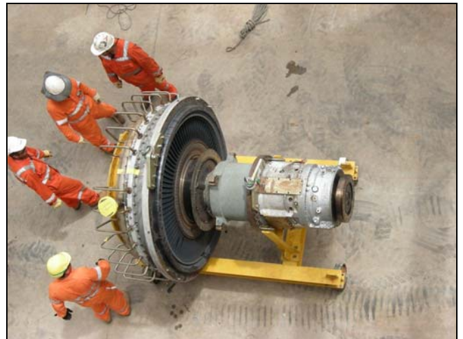
Figure 37. Power Turbine Module
