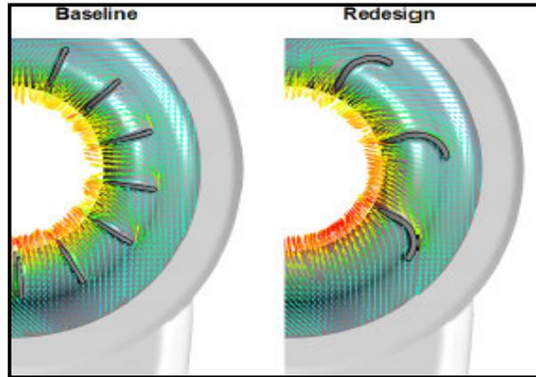
Figure 21. Side load vane CFD velocity profiles for Fourth Impeller
