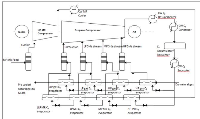
Figure 1. APCI C<sub>3</sub>-MR Refrigeration system for Trains 3, 4 and 5
