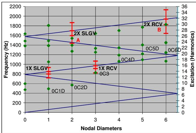
Figure 19. Fourth Impeller Interference Diagram
