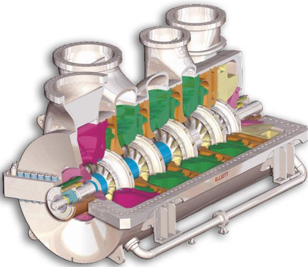
Figure 2. RasGas Train 3, 4 & 5 Propane Compressor
