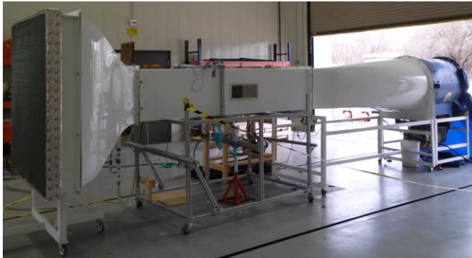
Figure 1. An open-loop wind tunnel is used to measure wet gas aerodynamic performance
