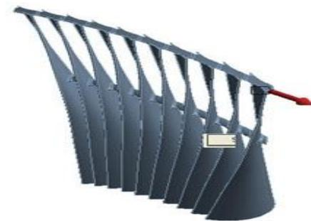
**Figure 18:** Blade pack stiffness evaluation
