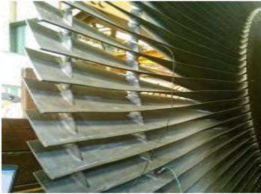
**Figure 2:** Pack of 8 blades with welded lashing wires
