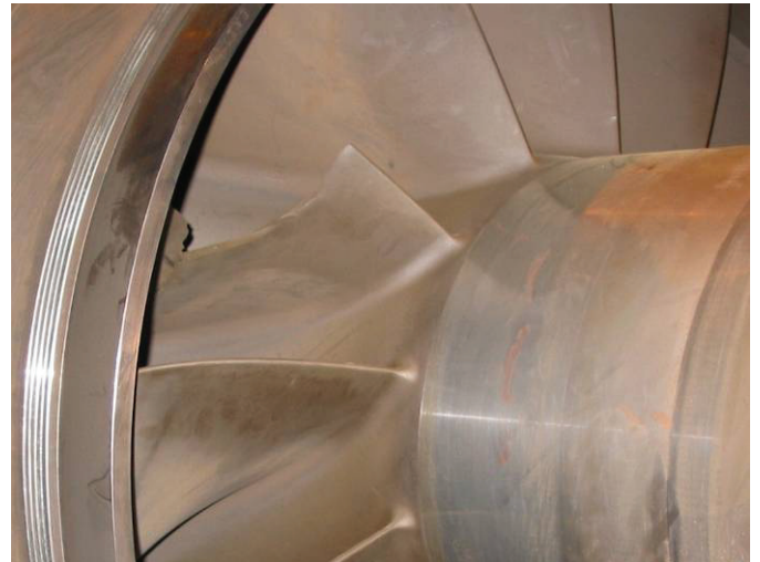
Figure 3. Fourth Impeller Released Piece at Blade Leading Edge
