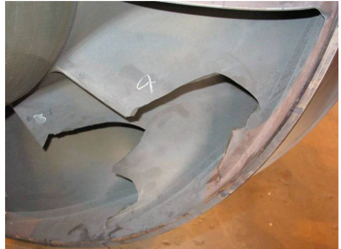
Figure 2. Fourth Impeller Released Pieces from Blade Leading Edge
