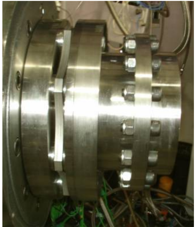
Figure 21. Test rig with drive bolt windage feature.
