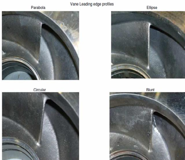
Figure 5: Cast Impellers with different leading edge profiles
