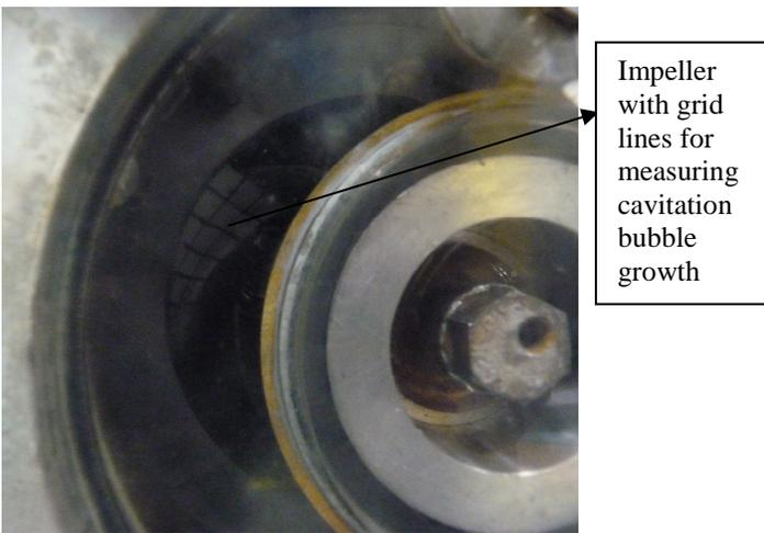
Impeller with grid lines for measuring cavitation bubble growth
