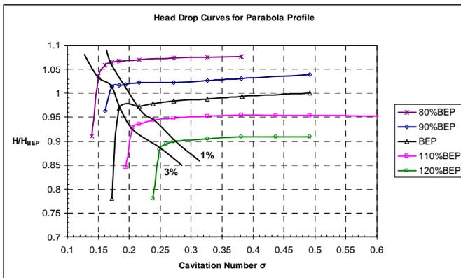
Figure 9: Head drop curves for Parabola profile at different
