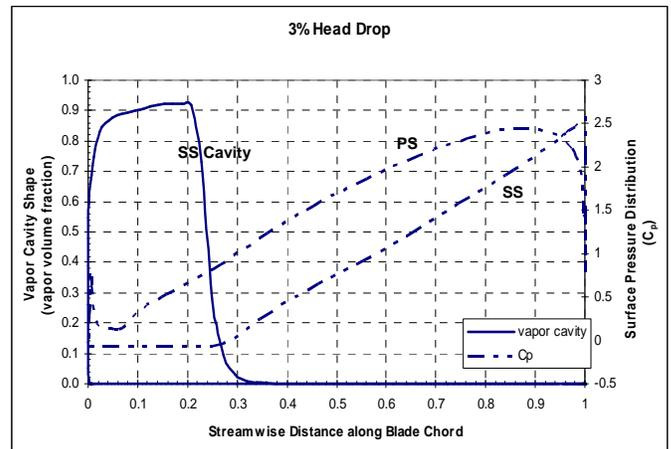
Figure 11: Vapor cavity shape and blade pressure distribution
