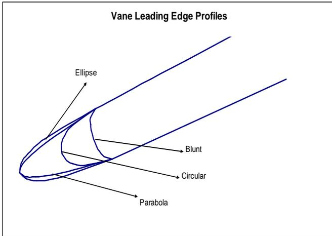
Figure 4: Different Vane Leading Edge Profiles
