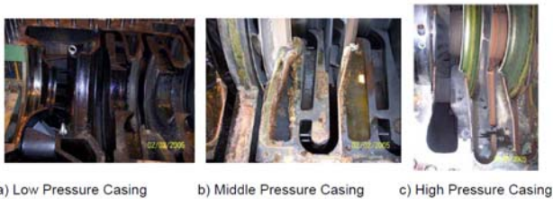
Figure 17: Typical Fouling Condition for Crack Gas Compressor
