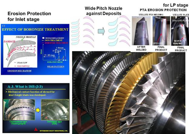
Figure 33 Improvement of Blade Integrity, Coating Application of Actual Blades and Additional Improvement for Anti-efficiency deterioration
