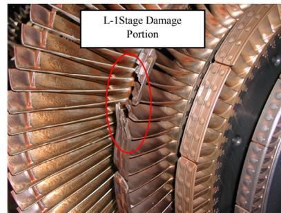
Figure 3 Typical Blade Damage of LP Section
