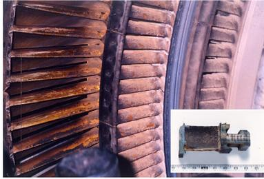
Figure 44 Deposit Condition of LP Section
