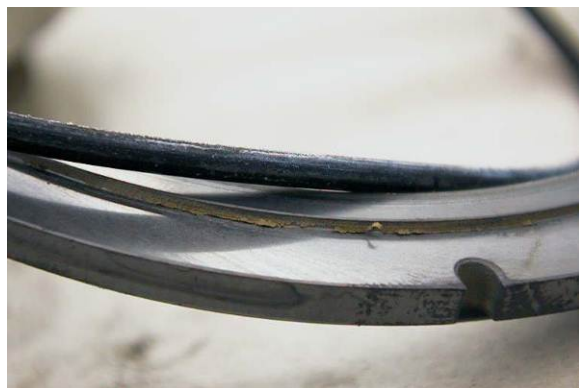
Figure 10: contaminated dynamic sealing element
