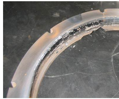
Figure 12: damaged seal faces → damage seal
