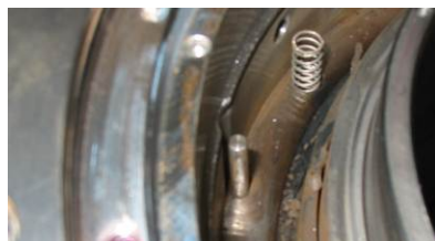
Figure 11: contaminated seal area behind stationary face
