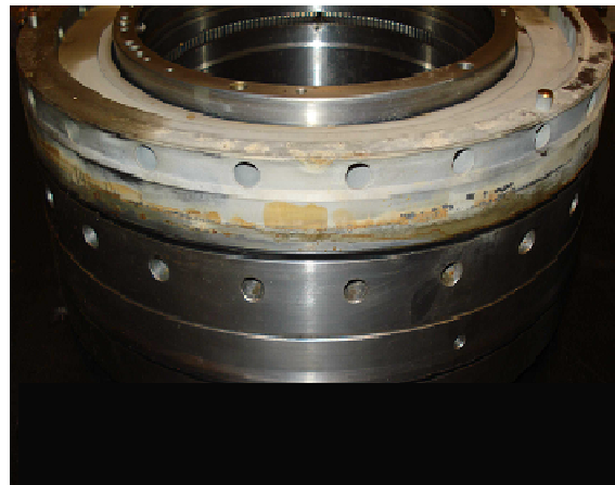
Figure 7. Salty deposit on gas seal housing.
