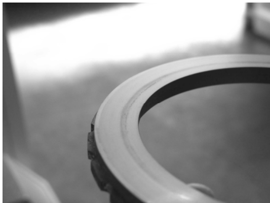
Figure 8. Scratched static seat.
