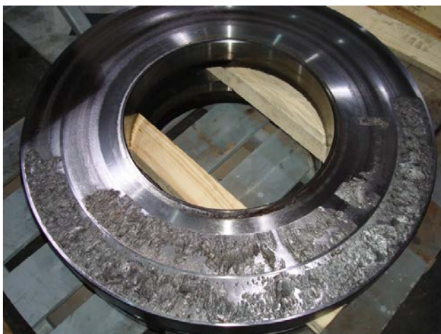
Figure 39b - Extruder Gearbox 2 Stages Tandem Bearing Outer Race - Damaged Condition
