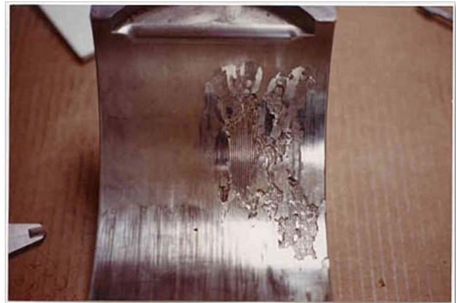
Figure 18 Wiping and fatigue/misalignment
