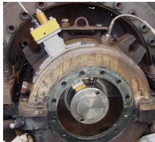
Figure 16- Typical Grounding Brush Installation (Sohre, 2010)
