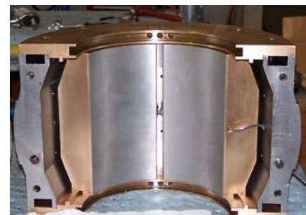
Figure 39 201A Bearing after 9 years in service
