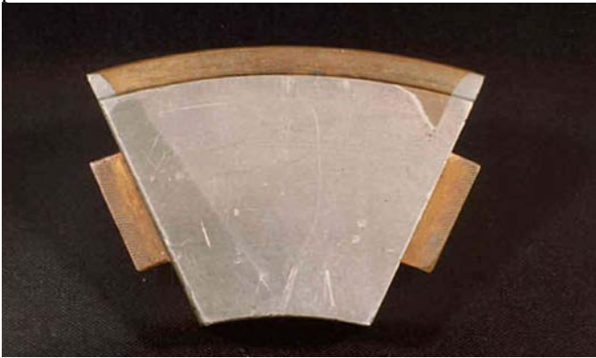
Figure 24 Thrust pad with electrostatic discharge damage
