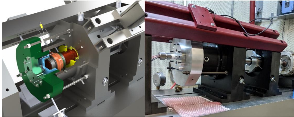
Figure 2: Left) Model of the mechanical seal test rig Right) Assembled view of the test rig.
