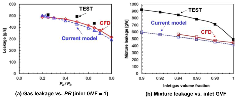
**Fig. 2** Current model predicted, CFD predicted, and measured [8] leakage for a PDS. (a) Leakage vs.  $PR$  (inlet GVF = 1), (b) Mixture leakage vs. inlet GVF (GVF = 0.9 ~ 1) and  $PR = 0.5$ . Clearance  $C_r = 0.20$  mm,  $L / D = 0.75$ ,  $P_s = 70$  bar, rotor speed 10 krpm.
