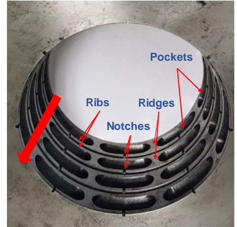
**Fig. 1 Photograph of typical pocket damper seal.**
