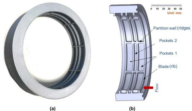
Fig. 2 (a) Photograph of test pocket damper seal (PDS), (b) Cut view of fully partitioned PDS.
