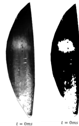
Figure 2 Overlap area between thrust collar and bull wheel highlighting locations of cavitation and turbulence
