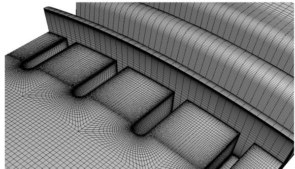
Figure 2: Computational grid for combined pre-swirl brake and labyrinth seal.
