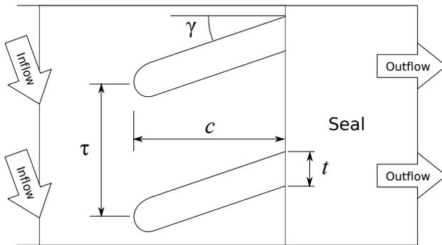
Figure 1: Design variables for pre-swirl brake: vane angle, thickness, chord length, and pitch.
