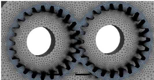
Fig 2. Detail of mesh showing gear engagement
