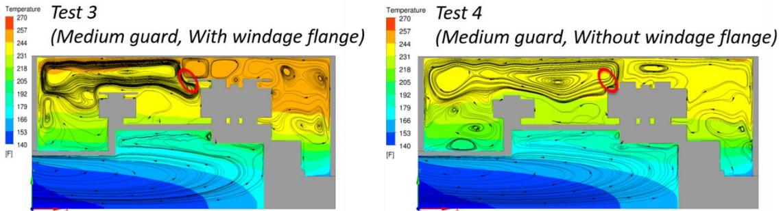
Fig 1. Comparison showing the effect of adding windage flange
