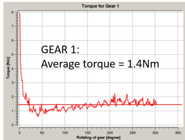
Fig 3. Evolution of torque value on gear 1
