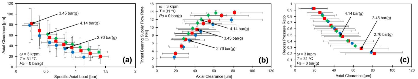
**Fig. 2. Water lubricated hydrostatic thrust bearing (a) axial clearance vs. specific load ( $W/A$ ), (b) supply flow rate vs. axial clearance, and (c) pocket pressure ratio vs. axial clearance. Operation at 3 krpm and bearing supplied with pressure  $P_s = 2.76, 3.45,$  and  $4.14$  bar(g). Water at  $3.45$  bar(g) feeds the journal bearings. Error bars indicate minimum and maximum clearances recorded on the face of the thrust bearing. Tests conducted at room temperature,  $31$  °C.**
