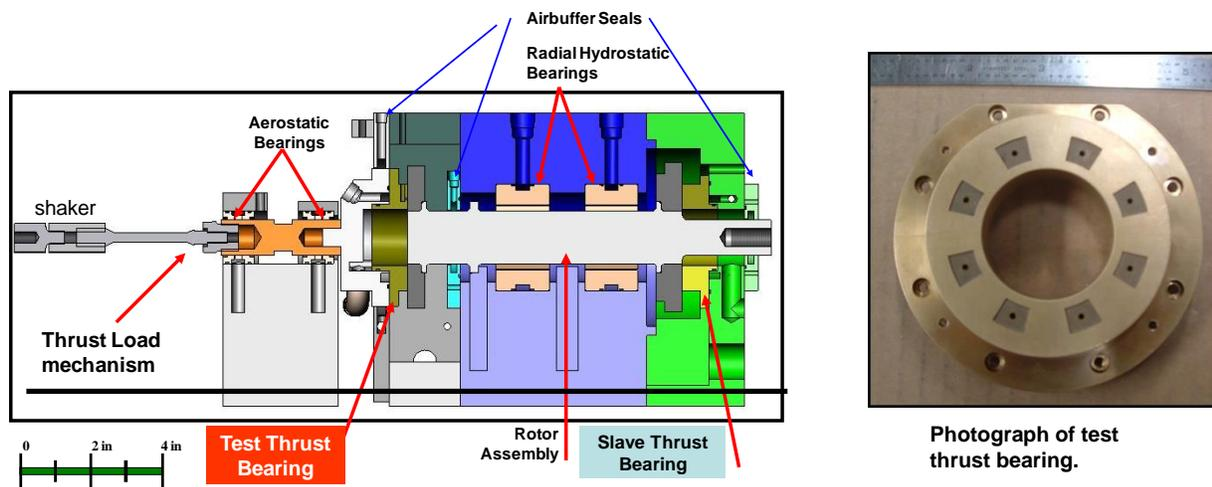
Figure 1. Schematic view of thrust bearing test rig [2].
